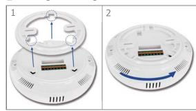
Wall Mounting (+ External Wall Box EWB-C150)
